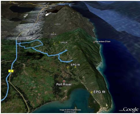
**Figure 4.8.** View west of prominent parallel west-southwest trending fault traces along south-facing slope of hills west of Petit Goâve Bay and Port Royal. Reconnaissance track marked in blue shows location of fault traverses west of Port Royal. Fault trace marked by push-pins labeled "EPG flt".
