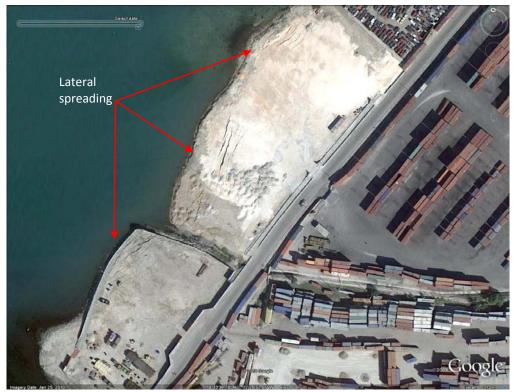
**Figure 6.20** Lateral spreading in the storage yards in the northern part of the port facility. Imagery courtesy of Google Earth. (18°33'40.23"N 72°20'52.33"W)
