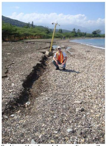
**Figure 7.4.** Cracking and lateral spread along coastline near village of L'Acul. (18°26'48.81"N, 72°41'11.92"W looking west).
