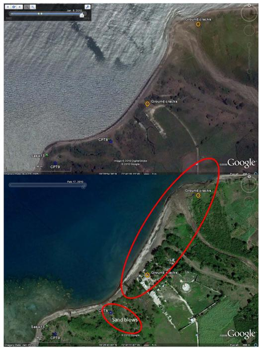
**Figure 7.3.** Pre- and post-earthquake images of coastline near village of L'Acul. Note in the lower, post-earthquake image the significant cracking subparallel to the coast and the arcuate slump in the northern end of the failure. SASW and DCPT testing was performed near several large sand blows located near the south end of the failure zone, as well as farther south outside of the failed reach. Imagery courtesy of Google Earth. Approximate center of image at 18°26'51.17"N, 72°41'11.06"W.
