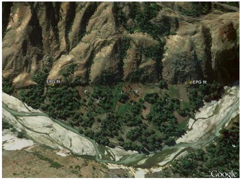
**Figure 4.2.** View south of prominent fault scarp crossing fluvial terrace on Momance River east of Fayette. Fault trace marked by push-pins labeled "EPG flt".
