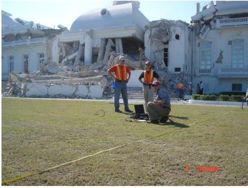
**Figure 5.9** The Presidential Palace lies within the heavily damaged zone noted above. Two SASW tests and one H/V Spectral Ratio test were conducted here (N  $18.543633^{\circ}$ , W  $-72.338905^{\circ}$ ).
