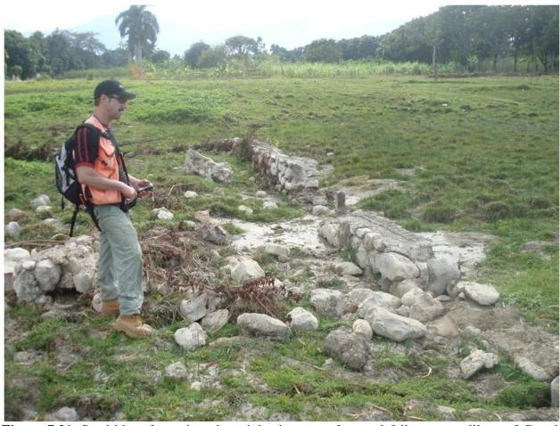
**Figure 7.21**. Sand blow formation along inland extent of coastal failure near village of Grand Goâve. (18°25'53.73"N, 72°45'37.65"W)
