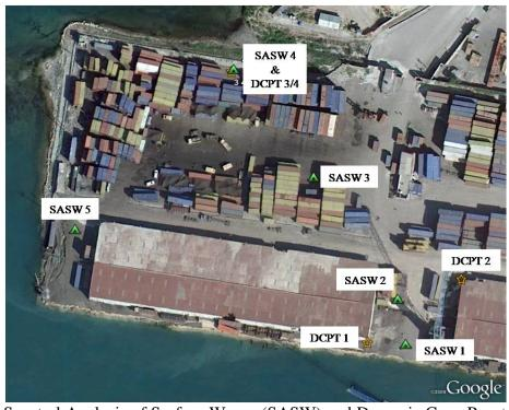
**Figure 6.26** Spectral Analysis of Surface Waves (SASW) and Dynamic Cone Penetrometer Test (DCPT) locations at the port in Port-au-Prince Haiti. Imagery courtesy of Google Earth. (Approximate long. and lat. of center of image: 18°33'27.09"N 72°21'03.51"W)
