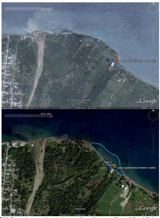
**Figure 7.16**. Pre- and post-earthquake images of coastline near village of Grand Goâve. Note in the lower, post-earthquake image the significant loss of coast as outlined in blue. SASW-11, DCPT-7, and DCPT-8 were performed just inland of the backscarp of the failed zone. Imagery courtesy of Google Earth.
