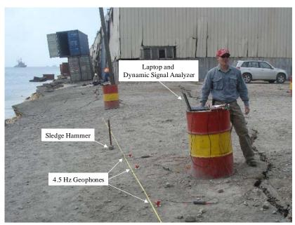
**Figure 6.27** Lightweight, dynamic equipment used to conduct SASW testing in Haiti. This photograph was taken at the location of SASW 1, facing West. (N18.556635°, W -72.350202°).
